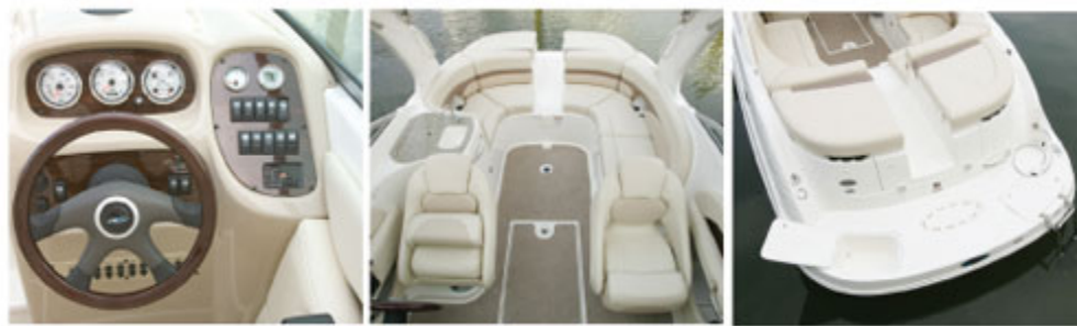
From left: The helm was fairly simple and included a four-in-one gauge, and rocker switches lined up on the right. In the cockpit, the snap-in carpet was plush and durable, a $580 option most buyers will want. Out on the swim platform the 225 SSi included a cooler, wash-down, stereo remote and a fold-down swim ladder. .....
